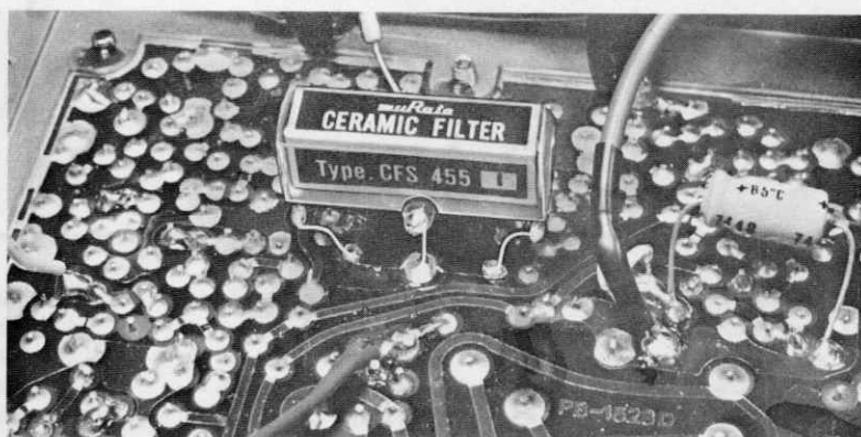
PHOTO "D" The new MuRata CFS-455-I filter is soldered to the PC foil so that it hangs upside down. Note the new position of the C5 substitution capacitor.
