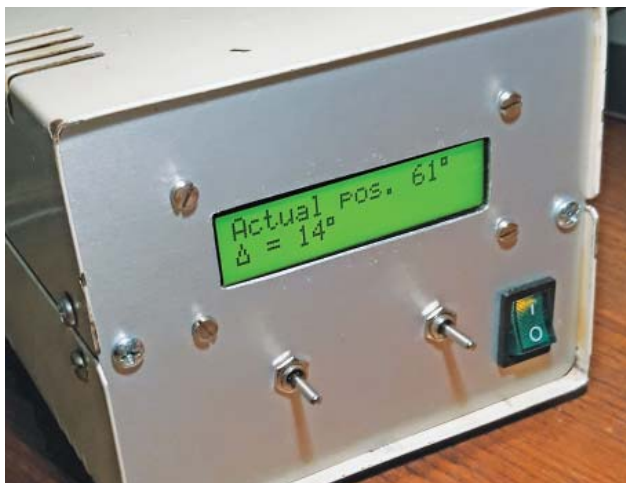
Figure 3 — The front-panel layout. The power switch is at the bottom right. The toggle switch on the left programs the direction (up or down). The toggle switch on the right starts the motor (up) or zeroes the rotator (down).
